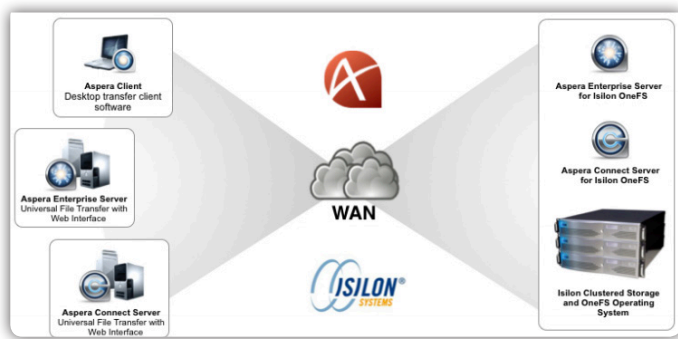
Figure 1: Aspera Enterprise Server and Connect Server Hosted on the Isilon Cluster
